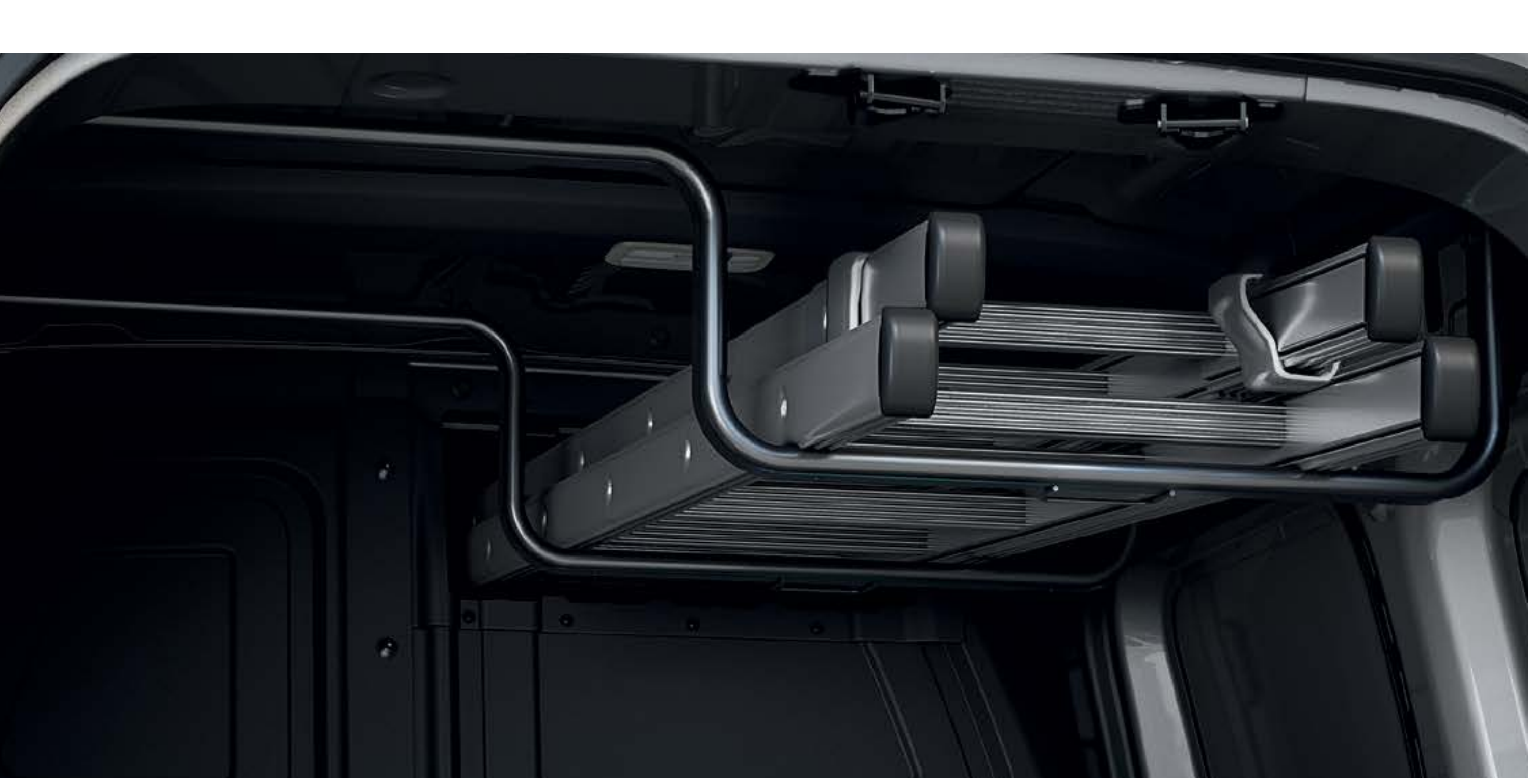
easy inside rack* with a load length of 2088mm and 2514mm
