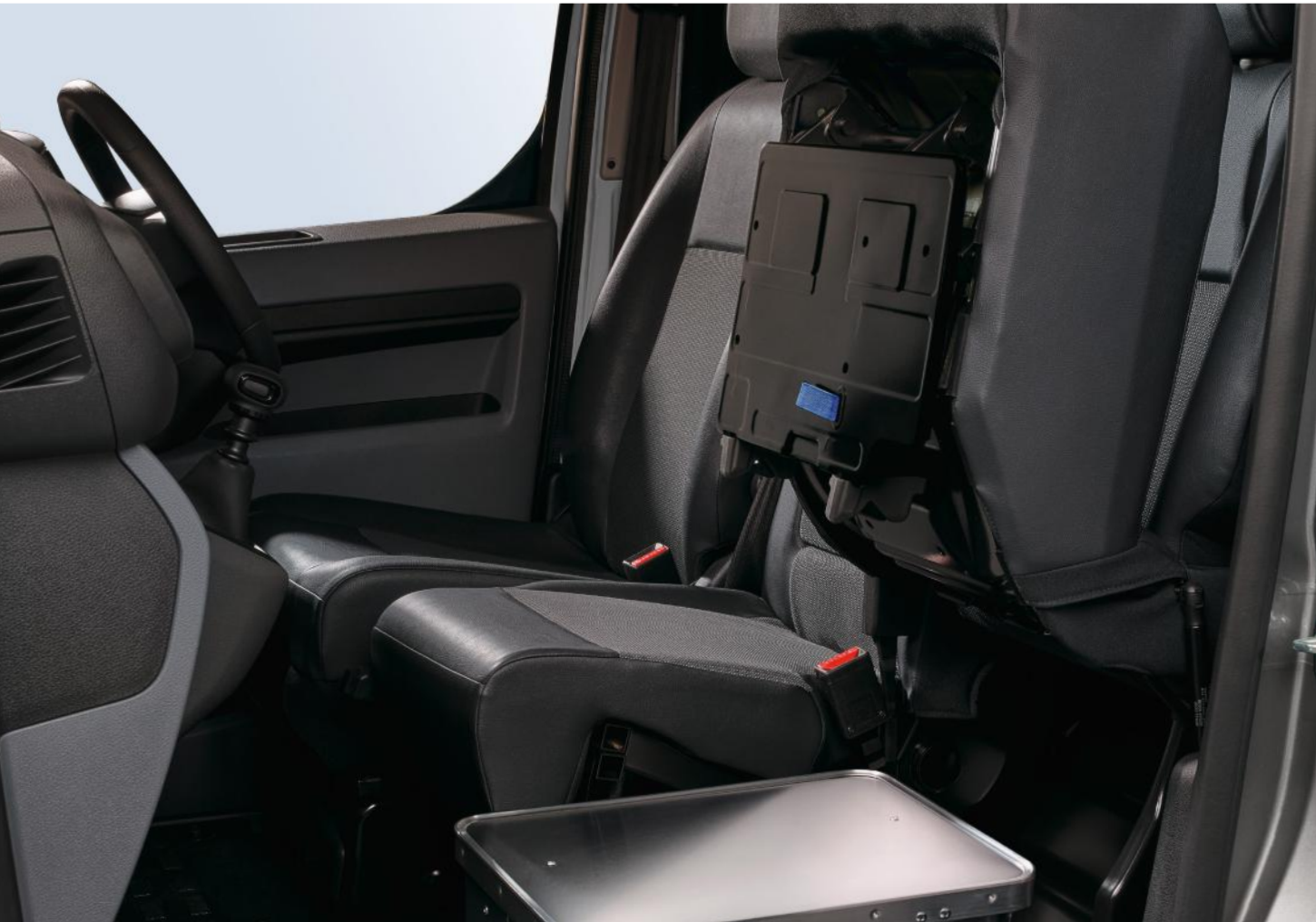
Load-through hatch within bulkhead.
