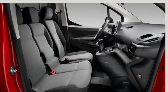
The central seatback can be folded down to access a pivoting table.
