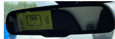
Electric Display in Rear Mirror: displays information including battery charge level and range
