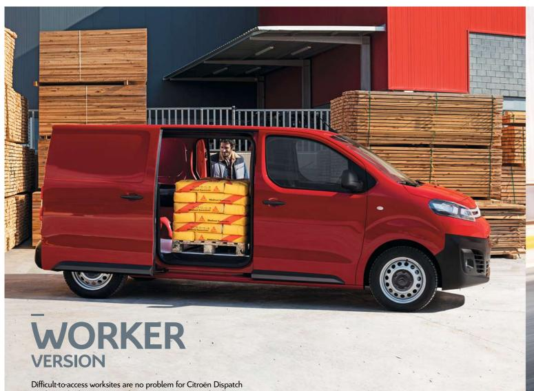
Difficult-to-access worksites are no problem for Citroën Dispatch Worker. Whether its cargo is heavy equipment or work colleagues, with Grip Control, a suspension raised by 20mm and a protective plate under the engine, this robust van will exceed your expectations. Available in M and XL sizes, it offers three seats at the front, the innovative Moduwork® seating and a payload of up to 1400 kg.
