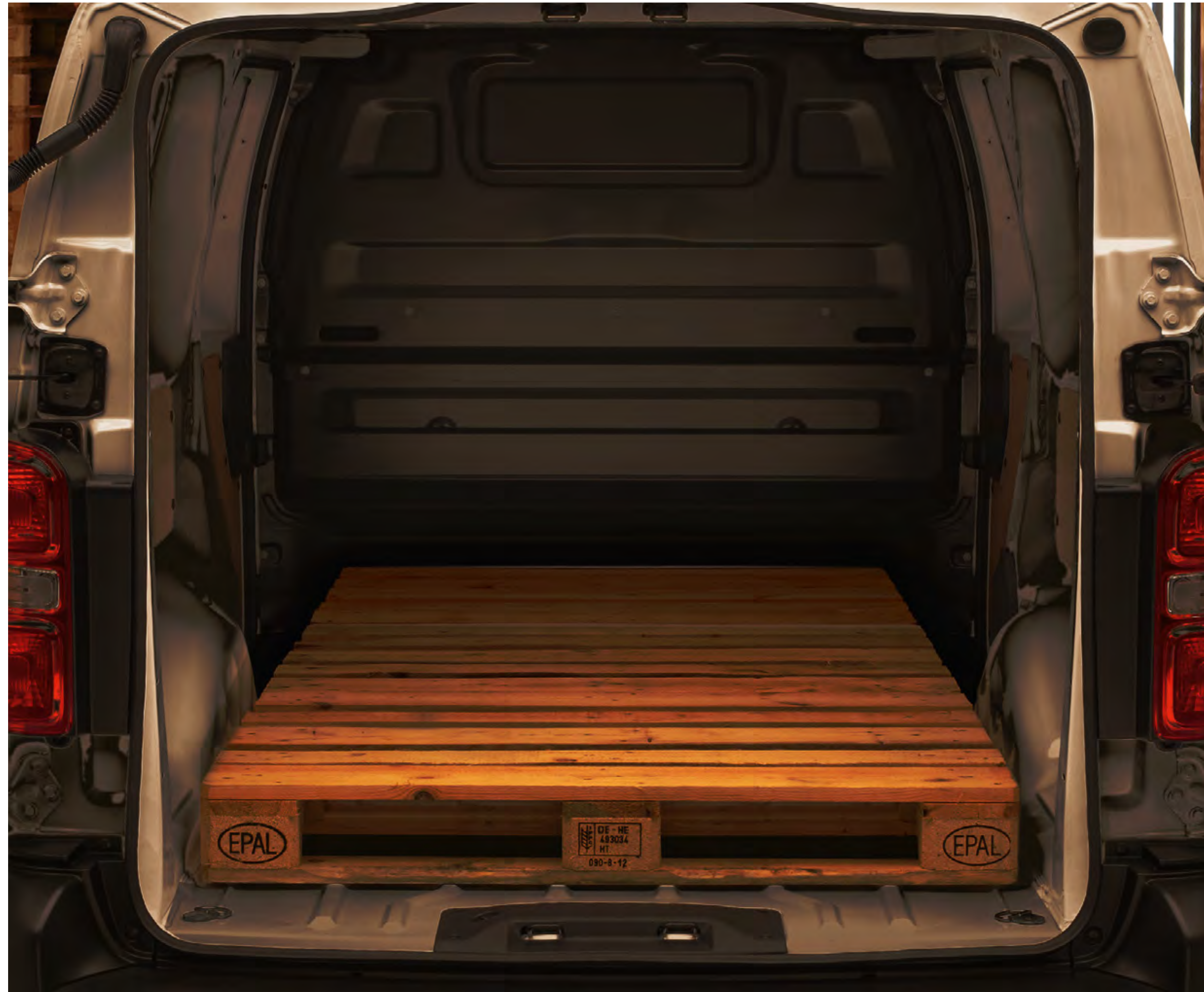
Full-height steel bulkhead.
