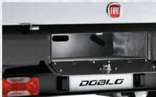
EXTERNAL COMPARTMENT WITH LOCK FOR STORING TOOLS UP TO 2 METRES IN LENGTH
