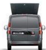
Rear roof window (opt. 585) available with 2-wing glazed or panelled rear door
