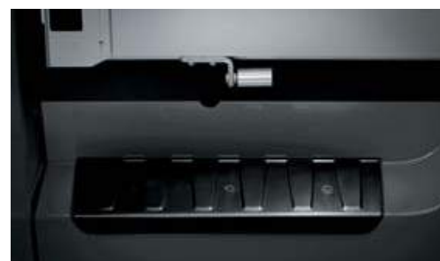
Hooks for securing loads on pole rack wall Side access steps
