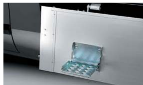
Internal steps folding into sideboards
