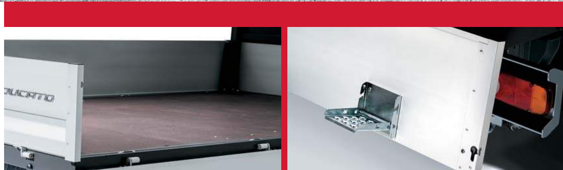
The load platform is lined with robust marine plywood.
