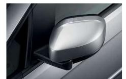
The BlueMotion's car-like aerodynamic wing mirrors. Available with optional body-coloured paint and optional electric folding function.
