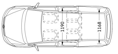
Please note: Vehicle drawings are not to scale. All dimensions in millimetres (mm), unless otherwise stated. The height measurements listed may vary by  $\pm$  50mm depending on model and equipment fitted.
