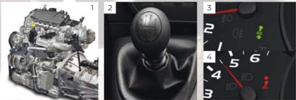
1) 2.3 LITRE DCI TURBODIESEL 2) SIX-SPEED MANUAL GEARBOX 3-4) GEAR SHIFT INDICATOR
