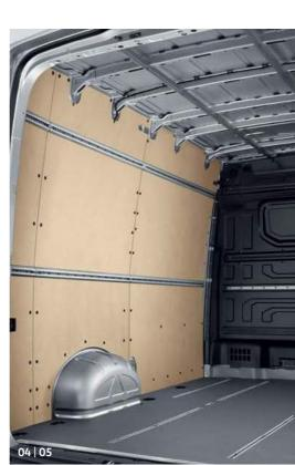
**02** Half-height plywood side lining.<sup>1</sup> The load compartment cladding made of 5mm thick rigid plywood panels is especially robust. It is fitted from the floor up to the load-lashing rails and is also highly durable.
