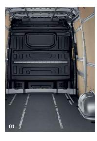
**01 Bulkhead – full-height without window.** A roof compartment above the driver's cabin is available upon request for the high roof variant and is a standard feature with the super-high roof.
