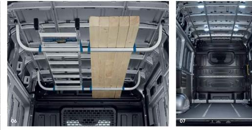
**06** Internal roof rack.<sup>1</sup> Enables easy transport of long objects. The two rails can be moved within the vehicle and adjusted to the length of the objects. They can also be removed when the roof rack is not needed.
